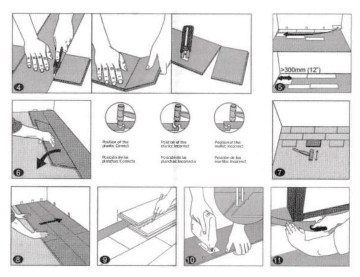
Step 4: Cut planks with a utility knife and ruler from the top side.
