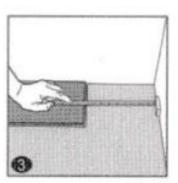
Step 1: Begin installation working from left to right, Insert Spacers at ends and edges where planks meet.
